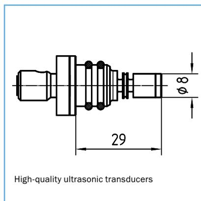
High-quality transducers are the heart of our intelligent measurement devices. All transducers are made of titanium, are hermetically sealed without a matching layer and wet gas protected. SICK transducers are subject to precise geometrical dimensional and impedance checks before they are matched pairwise to provide the utmost accuracy on each ultrasonic path for superior performance.
