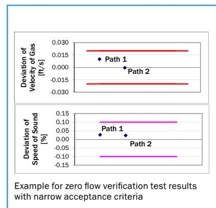
After assembly of the meter, a zero flow verification test is performed to verify proper transit-time measurement. Zero flow stability dominantly affects a meter's low-flow performance. The acceptance criteria for FLOWSIC600 zero flow verification exceeds the requirements from AGA9, and therefore ensures good low-flow performance.
