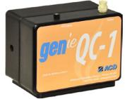
The **GENie QC-1** generates ammonia calibration gas using ampules of ammonia reactant. The concentration can be adjusted between 10 ppm and 500 ppm; each ampule provides 8 hours of calibration gas.
